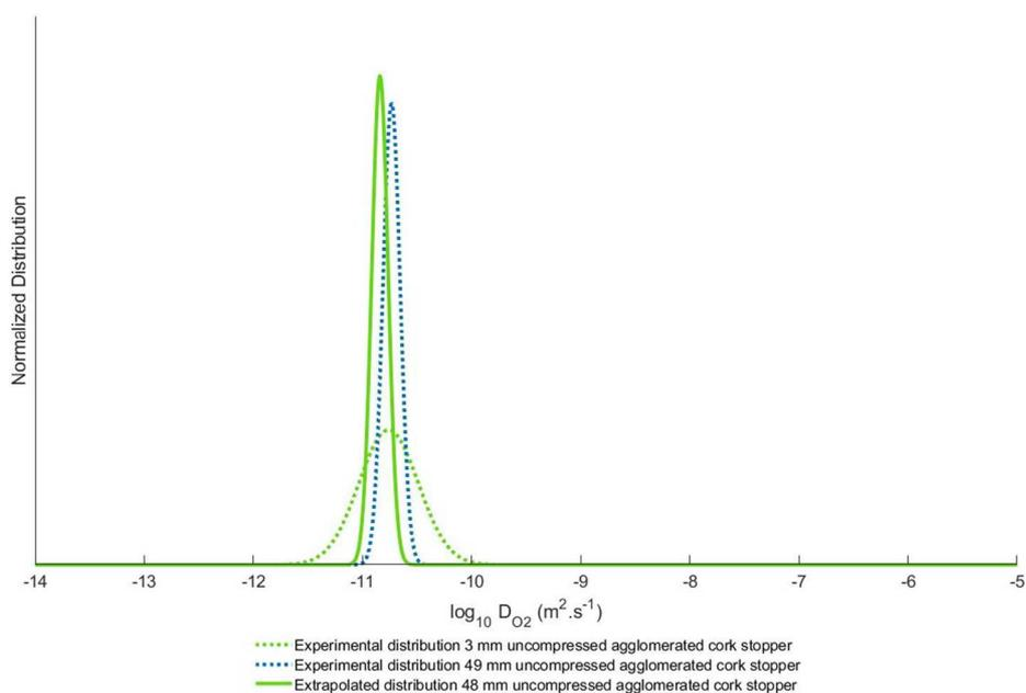
Figure 6 : Experimental distribution of effective oxygen diffusion coefficients measured on thin wafers of 3 mm or 6 mm thickness (--- green dash-dotted line), extrapolated distribution of the logarithm of the effective oxygen diffusion coefficient for a 48 mm length stopper, (- green line) and effective diffusion coefficient of oxygen for a 49 mm full-length stopper (-- blue dash-dotted line). A) Case of Natural cork (n=15), B) Case of Agglomerated cork (n=10).
