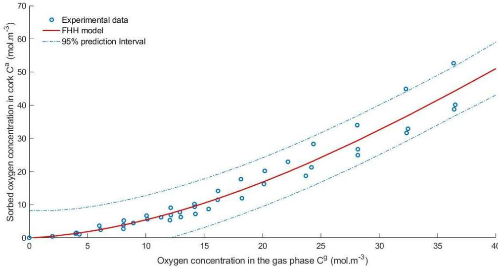
Figure 4: Sorption isotherm of oxygen on cork at 298 K for oxygen pressure ranging between 0 and 1000 hPa (o experimental data, - FHH model used to fit sorption data, -- 95% prediction interval); (data from Lequin et al.<sup>33</sup>)
