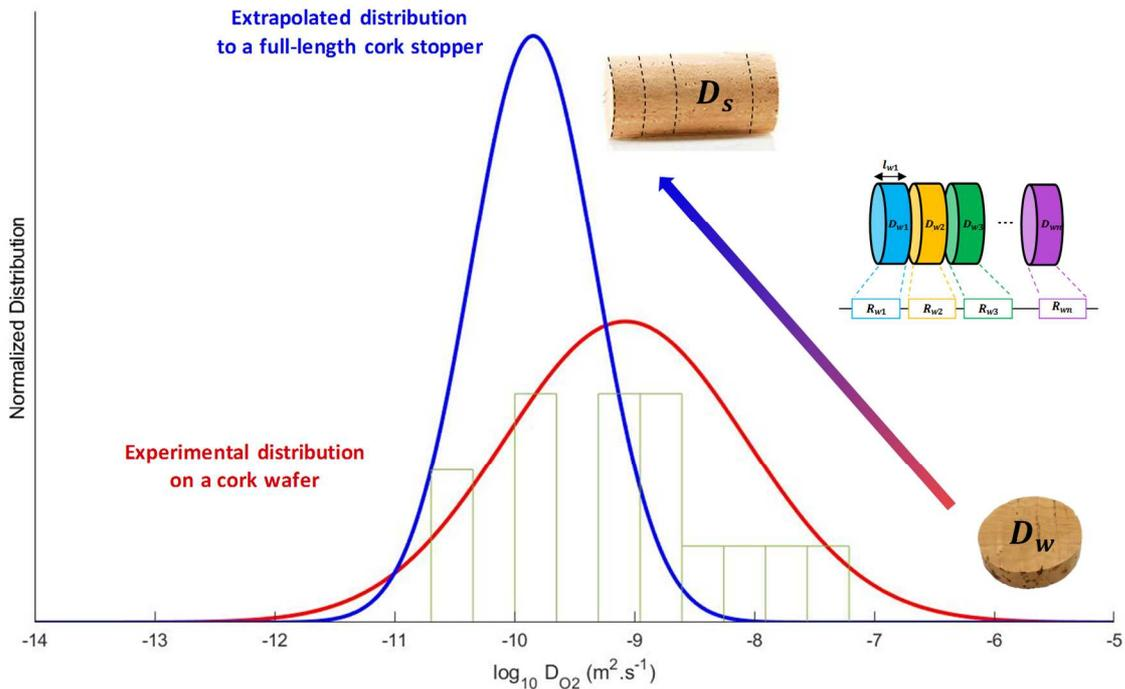
Figure 3: Experimental data (□ green rectangle) of the logarithm of the effective oxygen diffusion coefficient measured on cork wafers, corresponding experimental distribution (- red line), and extrapolated distribution (- blue line) of the logarithm of the effective oxygen diffusion coefficient of a full-length cork stopper, at 298 K.
