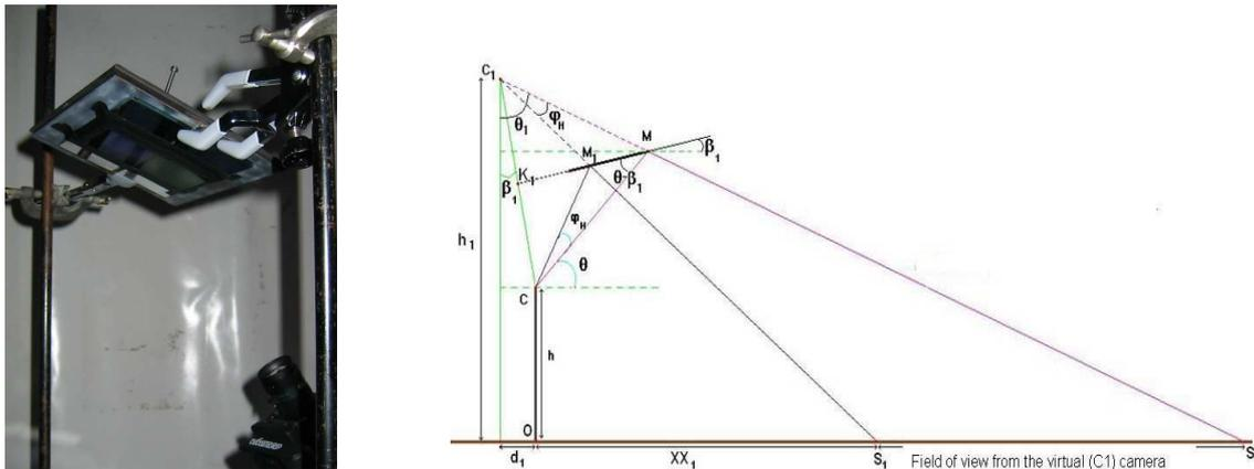
Fig. 1. a) The catadioptric viewer composed of a CCD monochrome camera with 2 mirrors placed above the camera. An interferential filter is fixed on each mirror. b) Optical model of the viewer system considering only one mirror (M1).
