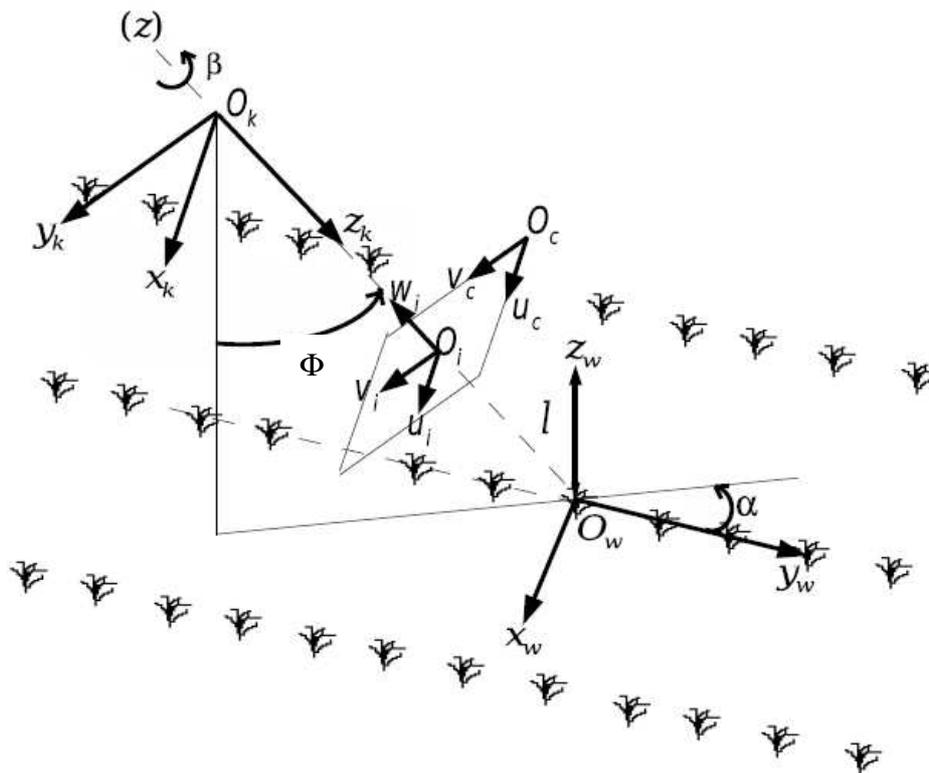
Fig. A1. Optical system with different coordinate systems : camera , image and real world.
