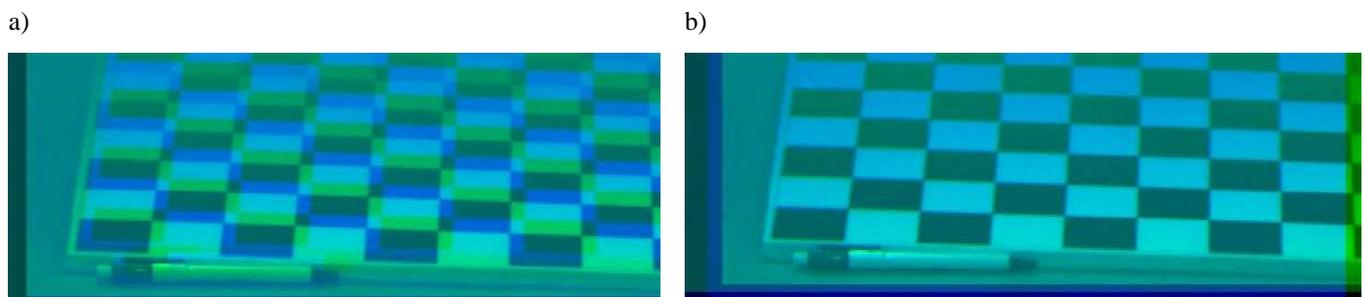
Fig.4: a) Superimposition of a pair of images splitted vertically from the vision system composed of a CCD monochrome camera with 2 mirrors (Green color: image from M1 and Blue color: image from M2) placed above the camera. b) Correction of a vertical offset (13pixels) and an horizontal offset (15pixels).
