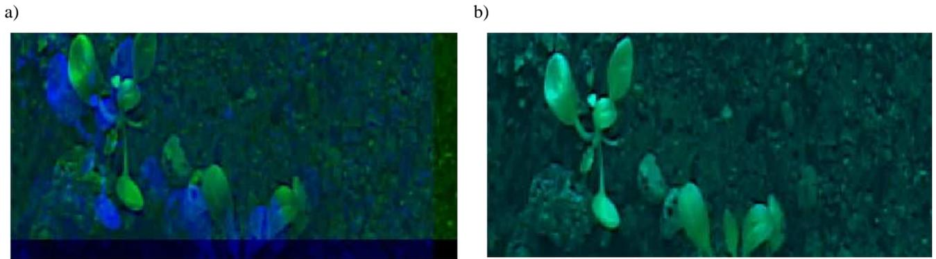
Fig.5: a) Superimposition of a pair of rectified images which have been splitted vertically from the vision system composed of a CCD monochrome camera with 2 mirrors (Green color : image from M1 and Blue color : image from M2). b) Correction with a vertical offset (13pixels) and an horizontal offset (15pixels).
